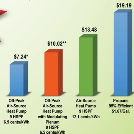
\* Outside temperatures fluctuate affecting the heat pump's efficiency. Efficiency and price per million Btus is estimated at 47 degrees F. Need additional heat like plenum heater in winter.
